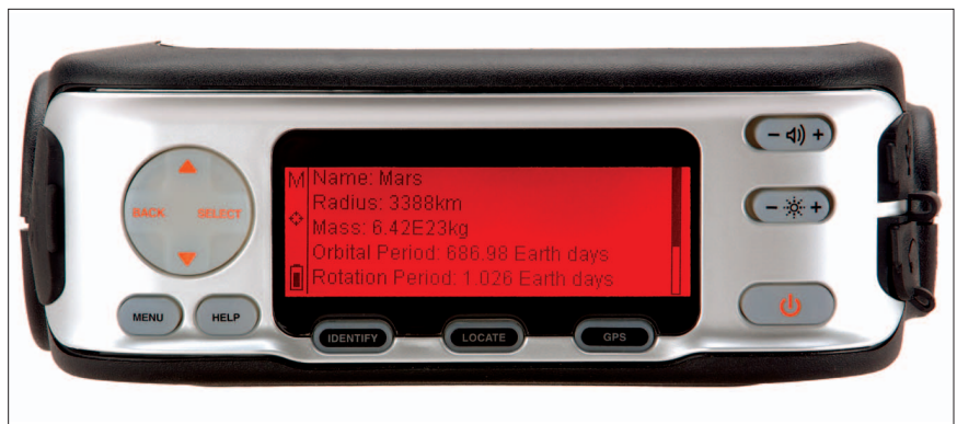
Figure 4. The SkyScout identifies and locates celestial bodies and provides text and audio information about them.
