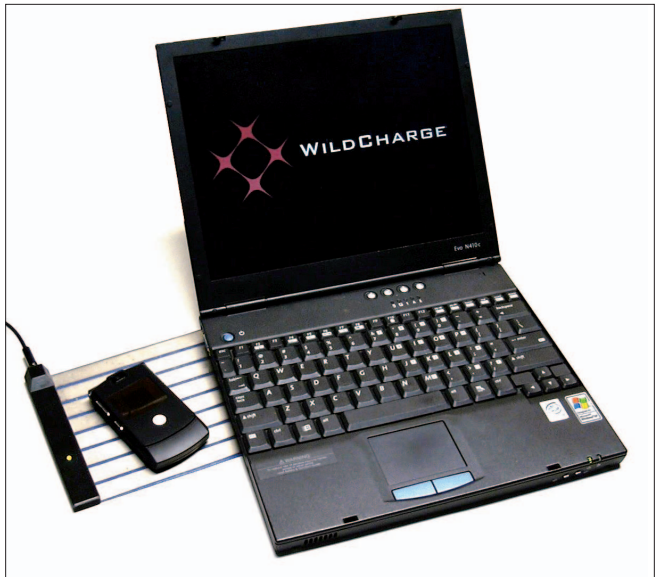
Figure 3. The WildCharger recharges mobile devices wirelessly, using electromagnetic induction.
